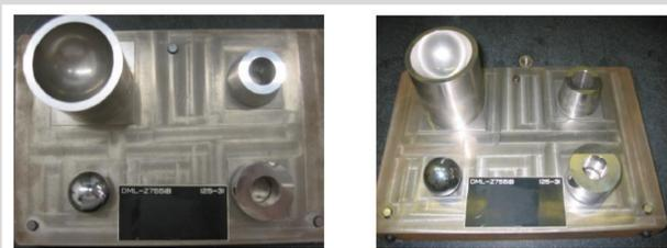
FIGURE 1. CMM TEST ARTIFACT USED IN PROFICIENCY TESTING
